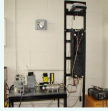
Moving bed reactor
